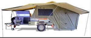
Kwik Awning with Vertical poles for wind & heavy rain conditions
